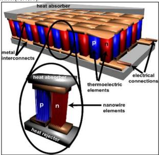
Fig. 2 Construction of a TEG
