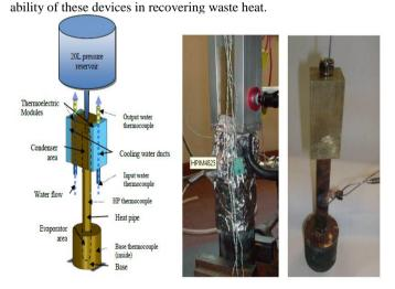
Fig. 5 Experimental set up dictating usage of heat pipe and cylindrical tank with thermoelectric modules.[4]
