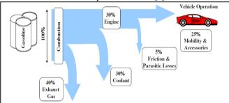
Fig. 1 Energy Distribution for an IC Engine [3]
