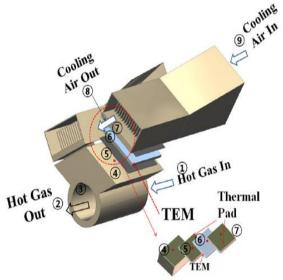
Fig. 11 Conductive TEG experimental system (TEGM 1) [8]
