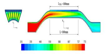
Fig. 9 Cross sectional temperature distribution
