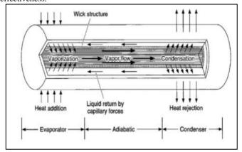
Fig. 3 Working of a Heat Pipe
